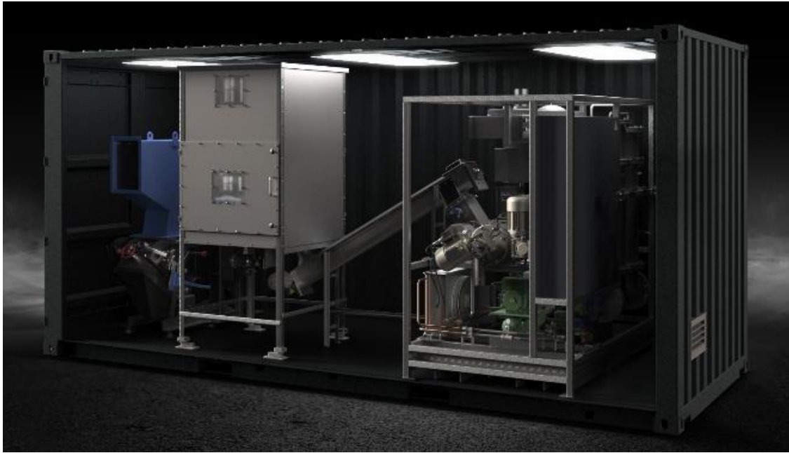
Figure 4: Image of the BioFabrik 1,000kg/day module with pre-processing on the left and pyrolysis on the right
